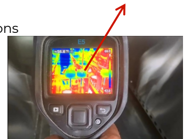
Thermal image of Potted parts curing at 60°C inside the oven
